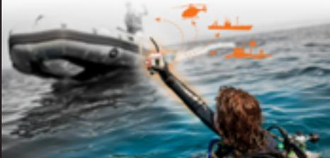
automated distress signal by pushing and holding the red button for three seconds. In this situation all modern VHF marine radios within range will receive an automated distress signal alarm and your exact coordinates will be visible on the readout of their marine VHF radio. In automated distress mode the range is double the range of normal voice communication.
